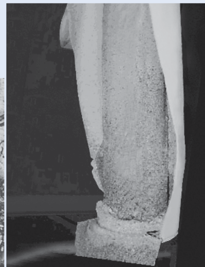
Cutaway of the element from an E-coat tank filtration after being in service for eleven weeks
